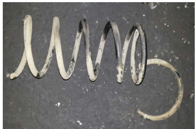
Fig.1.1 Broken Helical Coil Spring
